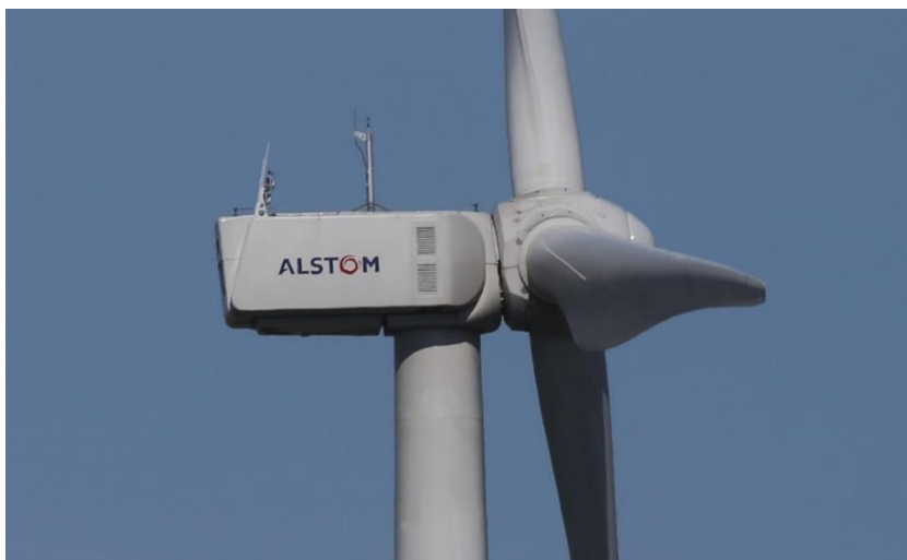
Figura 152. Aerogenerador Alstom ECO 122/2700. Tomado de: (wind-turbine-models.com, 2022)
